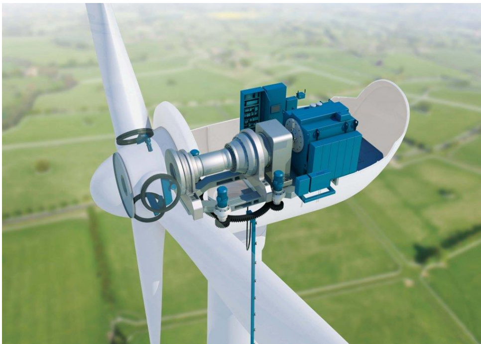
Figure 81: Nacelle of a wind turbine where the AFPS is installed
