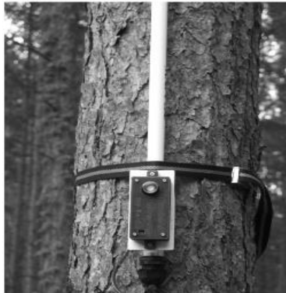
Figure 32: Hydrogen sensor mounted to a tree during an experiment done in Humboldt University in Berlin, Germany. [9]
