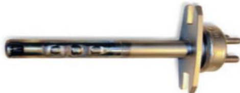
Figure 78: Thermocouple used in Siemens SGT [54]
